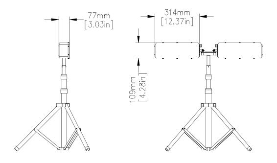
• The mast height is 1.6m ,2m,2.8m ,3.5m is for optiaonal or customized
